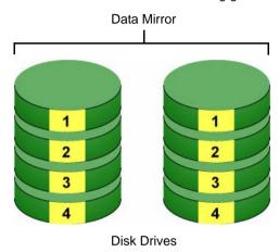
Figure 2. RAID 1 Mirrors identical data to two drives
